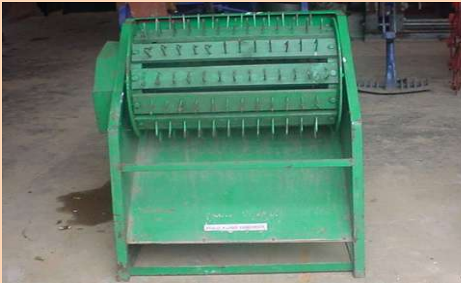
Fig : Paddy Operated Paddy Thresher
